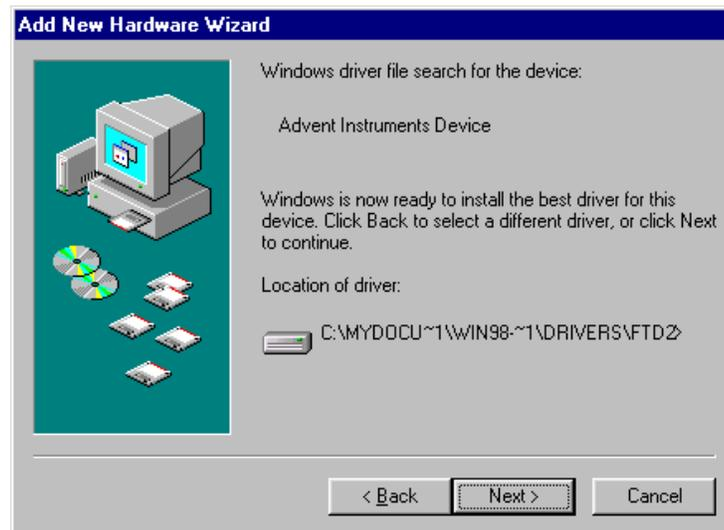
Once the installation is complete, the AI-7280 will be ready for use. The name for the USB driver is "Advent Instruments Device" so that when viewing the Control Panel's 'Device Manager' window.
